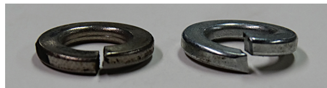
Fig. 3 — Stainless steel lock washer removed from the assembly (left) compared to a new lock washer (right).
