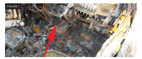
hile operating his vehicle, the insured smelled smoke, stopped the vehicle and opened the hood to assess the situation. He noticed a glowing wire generating smoke. Suddenly, a fire developed in the instrument panel of the occupant compartment, causing a total loss of the vehicle.
